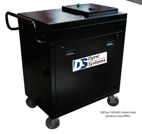
Dyne Systems has a family of Closed Loop Cooling Centers (CLCC), each sized to handle the heat rejection typically required for engines that are of 200 hp, 500 hp, 800 hp, 1,250 hp and 2,500 hp (149 kW, 373 kW, 597 kW, 932 kW and 1,864 kW). The CLCC allows you to use a glycol-based coolant to regulate an engine coolant circuit temperature while cooling the CLCC with the facility process water.
