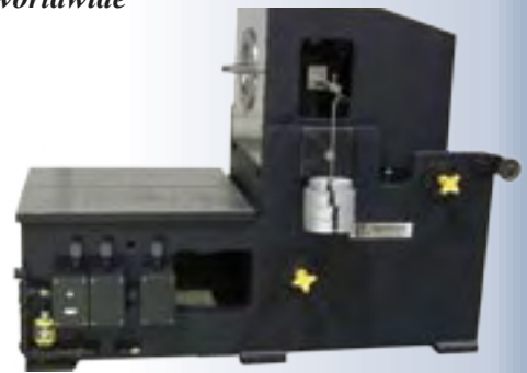
Vertical/Horizontal tilt stand for testing engines or motors up to 75hp
