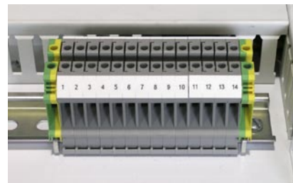
Figure 4. The terminal blocks on the 15 and 25 Amp power amplifiers will accept wires as large as 10ga.
