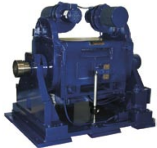
400hp Trunnion mounted, blower cooled AC Dynamometer with 0-1200 RPM constant torque range, 1200-3600 RPM constant HP range, and 3600-5000 RPM decreasing HP range (300HP)
