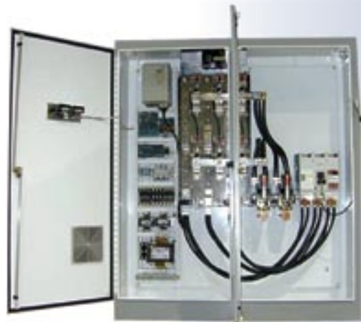
Double door, floor-mounted regenerative DC drives Shown with optional DC contactor. Rated from 1300 to 2000 Amps, and maximum 600HP at 250 VDC Armature voltage or 1300HP at 500 VDC Armature voltage
