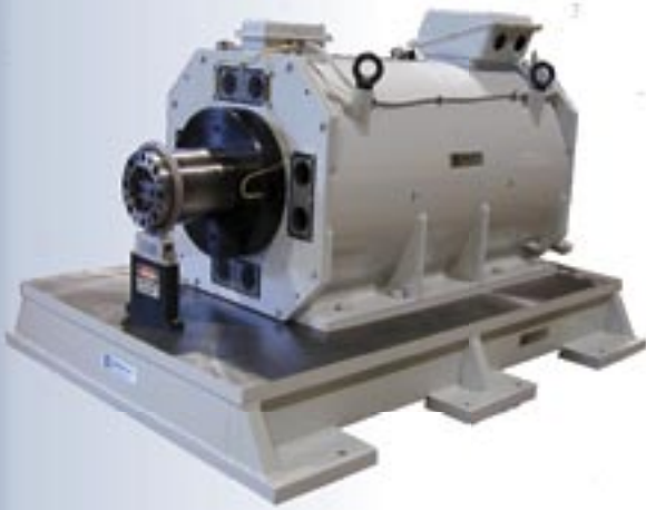
600hp Foot-mounted liquid cooled AC Dynamometer with 0-450 RPM constant torque range, 450-900 RPM constant HP Range, and 900-2500 RPM decreasing HP range (400HP)
