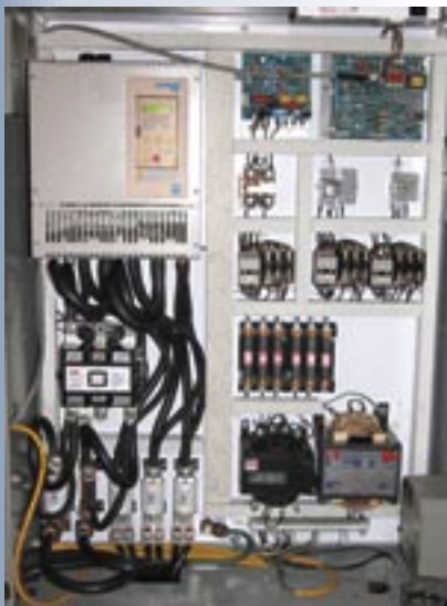
Single door, floor-mounted regenerative DC drives Shown with optional DC contactor. Rated up to 850 Amps, and maximum 300HP at 250 VDC Armature voltage or 600HP at 500 VDC Armature voltage
