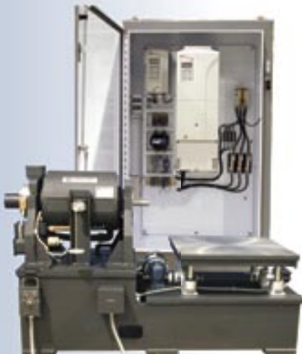
50hp trunnion mounted, liquid-cooled AC Dynamometer with 0-2200 RPM constant torque range and 2200-6000 RPM constant HP range, in an adjustable-height test stand.
